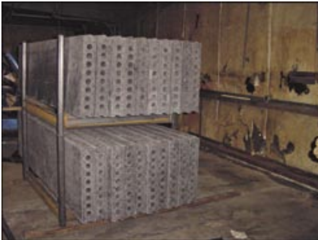
Quick setting concrete is used to manufacture panels made with a series of round voids to greatly reduce panel's weight and enhance insulation and strength.
