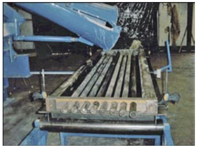
Unusual forms of steel are conveyerized to locations beneath pouring troughs to receive the unique mixture of concrete, special ingredients plus encapsulated wood fibers.
