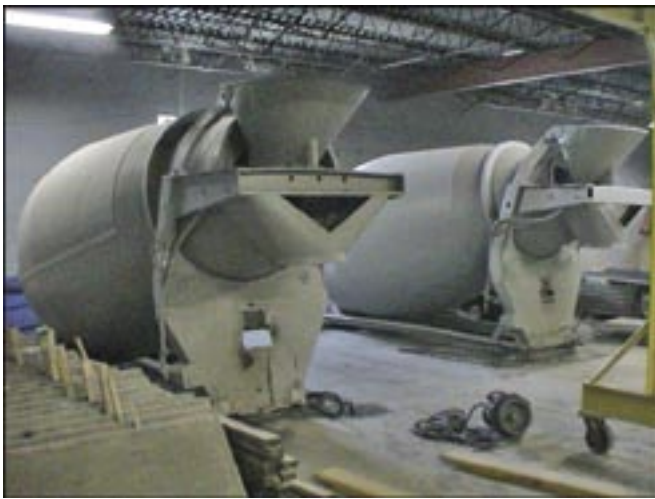
Massive mixers are used to create the concrete ingredients for the First National Panel Construction products.
